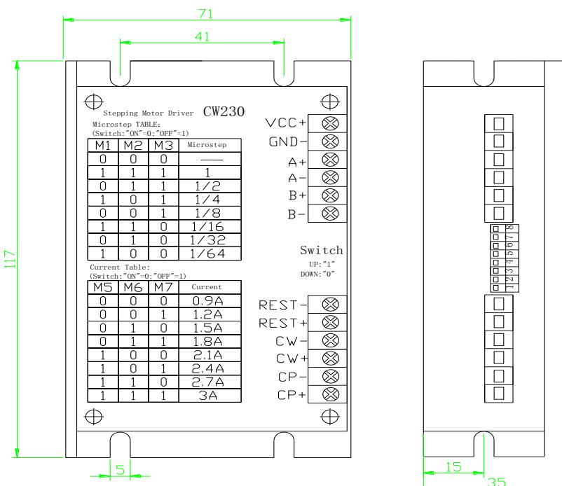
**CW230 2-Phase Mircostepping Motor Driver Photo for CW230**
